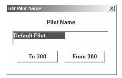
Copy the active pilot's name from the 302 by pressing [From 300]. Type in a new pilot's name and send it to the 302 by pressing [To 300]. **The Utility program deletes ALL pilot names entered via the 303-NAV Display!**
