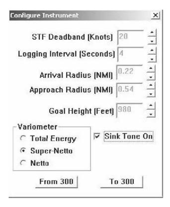
The current instrument configuration is automatically shown if the DDV is connected and turned on. You can also use "From 300" to see its settings. Use "To 300" to send the settings to the instrument.
