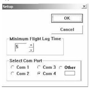
The serial datacom port on most computers is configured as COM1. Try COM2 if COM1 doesn't work. PC card serial port adapters and USB serial port adapters are available for laptops that do not have a built-in serial datacom port. These devices are typically configured as COM4 or higher.
